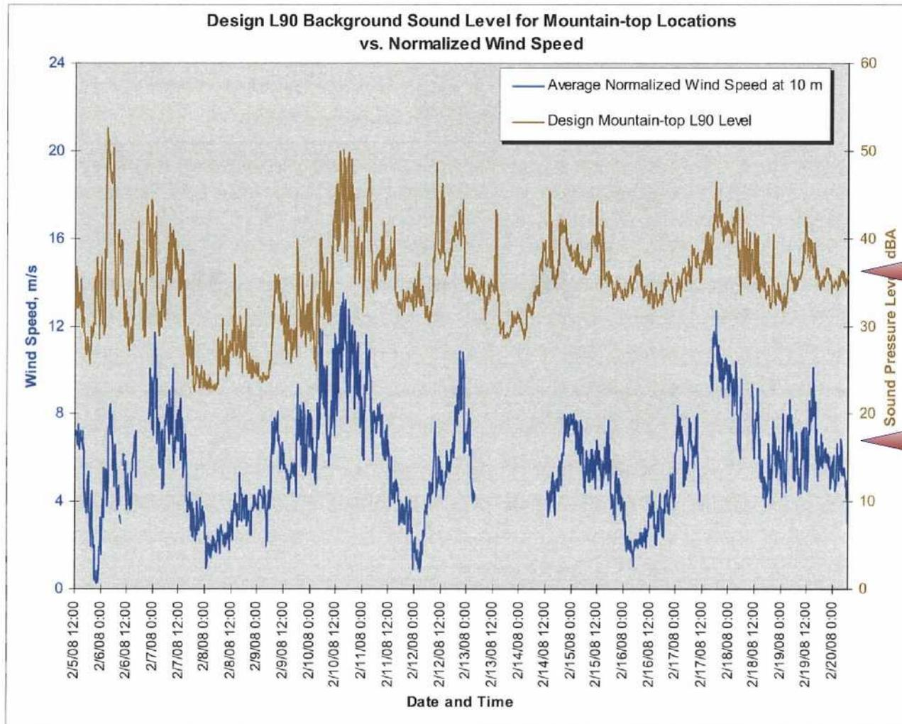
Figure 2.5.7 Design Mountain-top Sound Level Compared to Wind Speed
