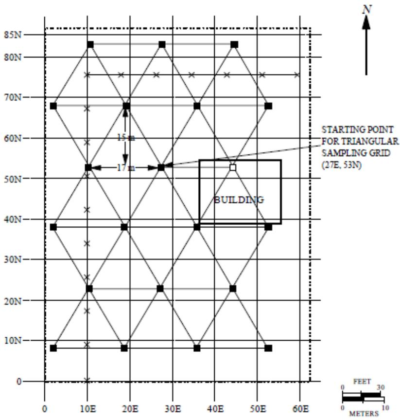
Figure 2a. Sampling Array recommended by MARSSIM (MARSSIM, 2000)
